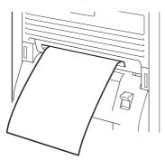
**8** Remove the paper from the back side of the cleaning sheet (the side without illustrations).
